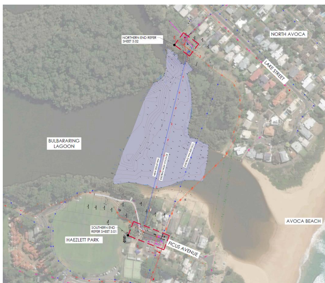
Figure 2: Avoca lagoon crossing Horizontal Directional Drilling (HDD) setup areas
