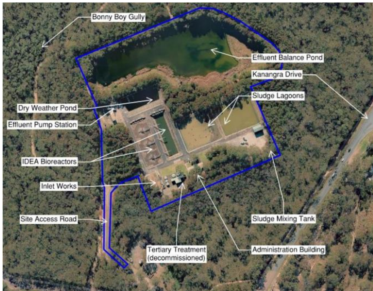
Figure 30: Gwandalan STP site layout
