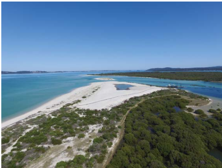
Photo: The dredge in operation during September and the beginnings of the newly created channel. The big pond of water is where the dredge deposits the sand pumped from the channel - as the water soaks away, sand is left behind. Photo courtesy of Rick Wraight, Tea Gardens Real Estate.
