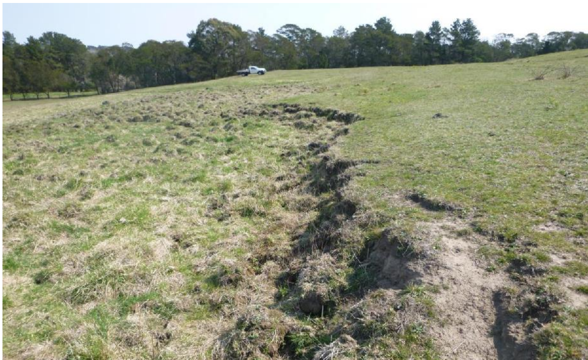
Photo 7: View looking northwest across the active scarp in the lower-middle part of the hillside in the northern part of the site.
