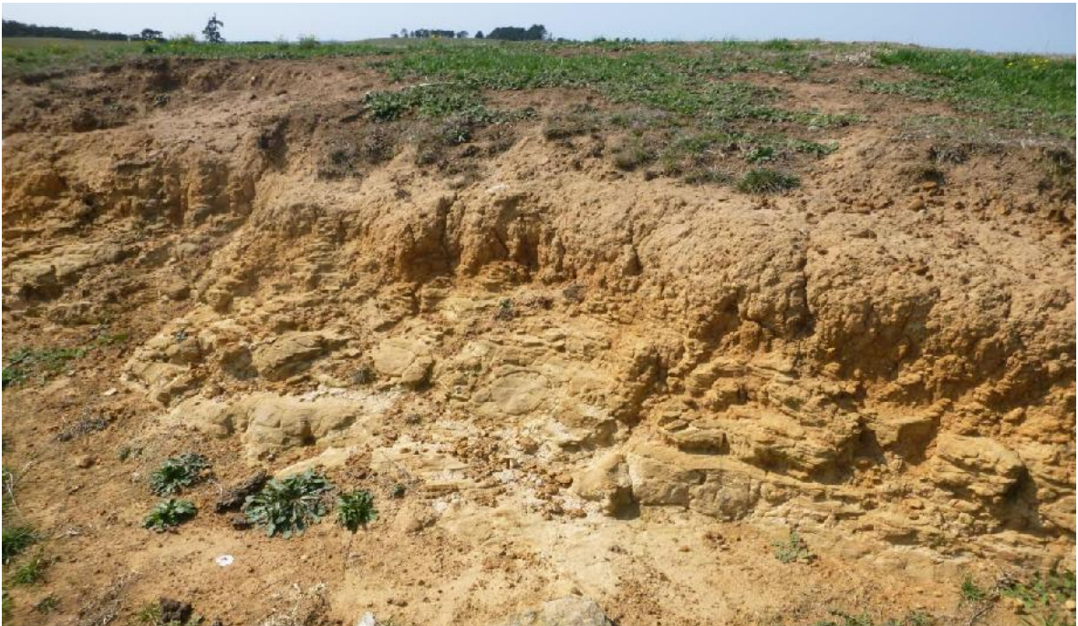
Photo 12: View looking at fine-grained sandstone exposed in a cutting in the eastern part of the site.
