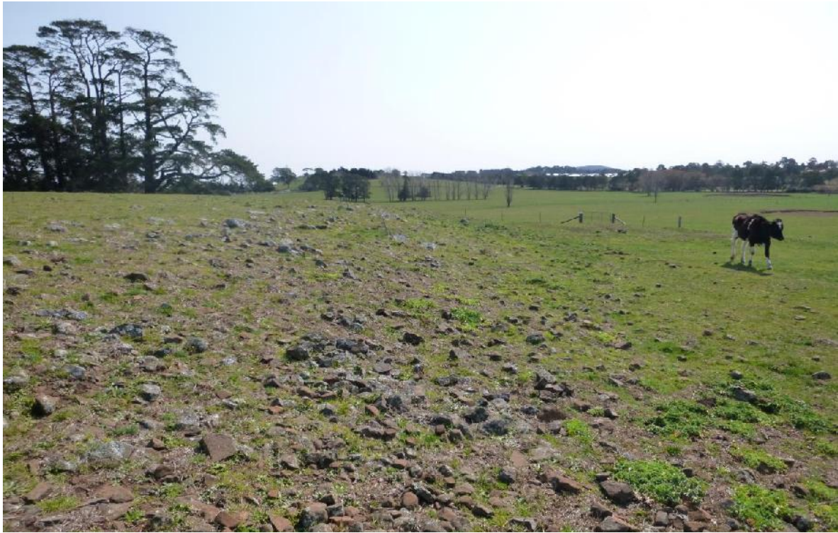
Photo 14: View of looking at igneous cobbles exposed at the surface along a low natural batter in the southern part of the site.
