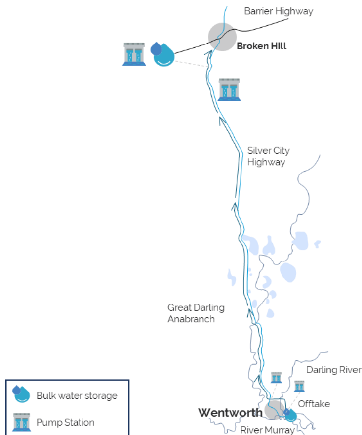
Figure 1 The WaterNSW Pipeline transports water from the Murray River to Broken Hill
