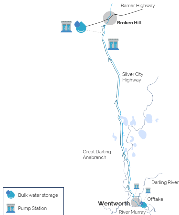
Figure 2.1 The WaterNSW Pipeline transports water from the Murray River to Broken Hill
