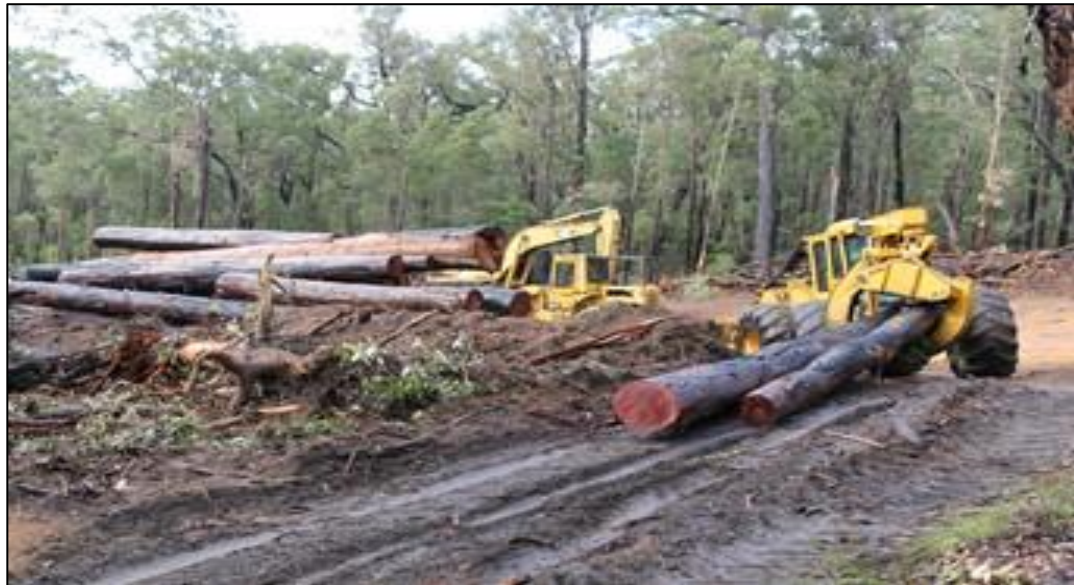
Plate A14: Western Australian Jarrah harvesting – note logs are ‘bark on’ and of mixed log quality with little log grade segregation
