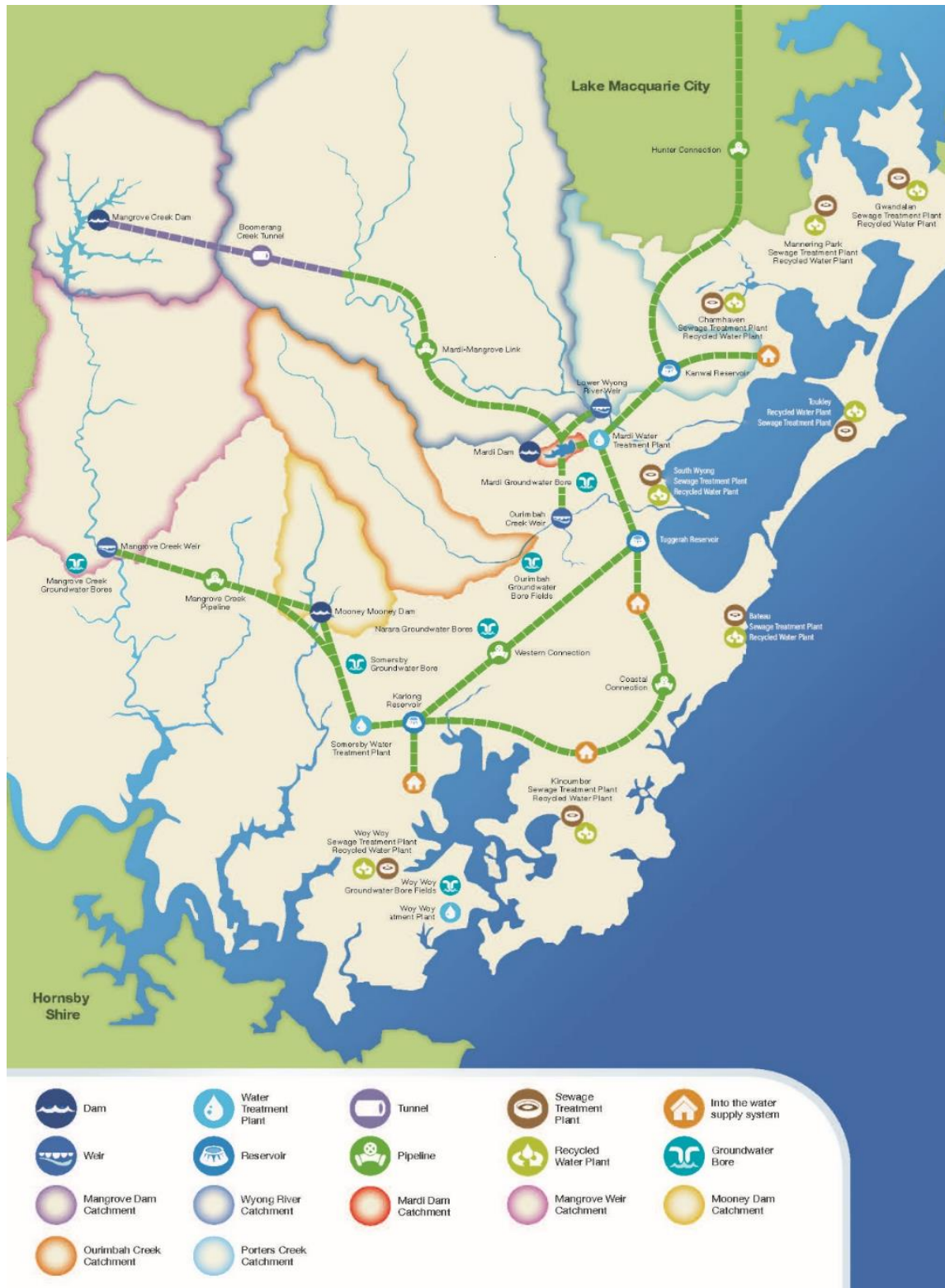
Figure 2-1 Schematic of Council's water and sewerage assets
