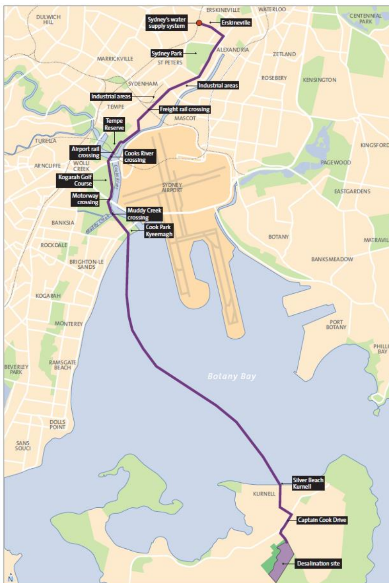
Figure 2-1 Pipeline Route from Kurnell to Erskineville
