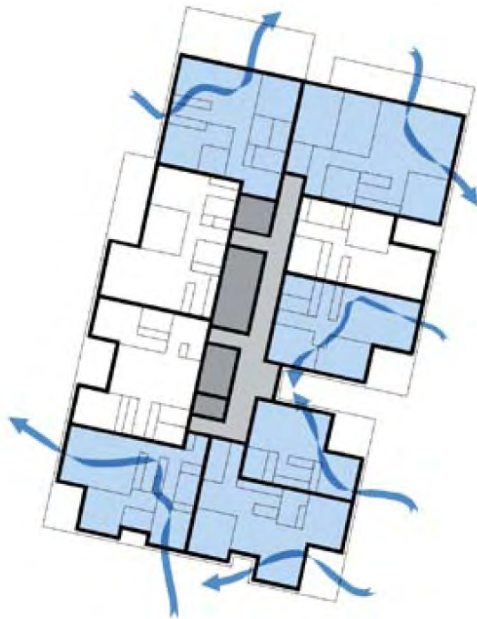
Figure 22 – Cross ventilation of typical Building 1C floor plate
