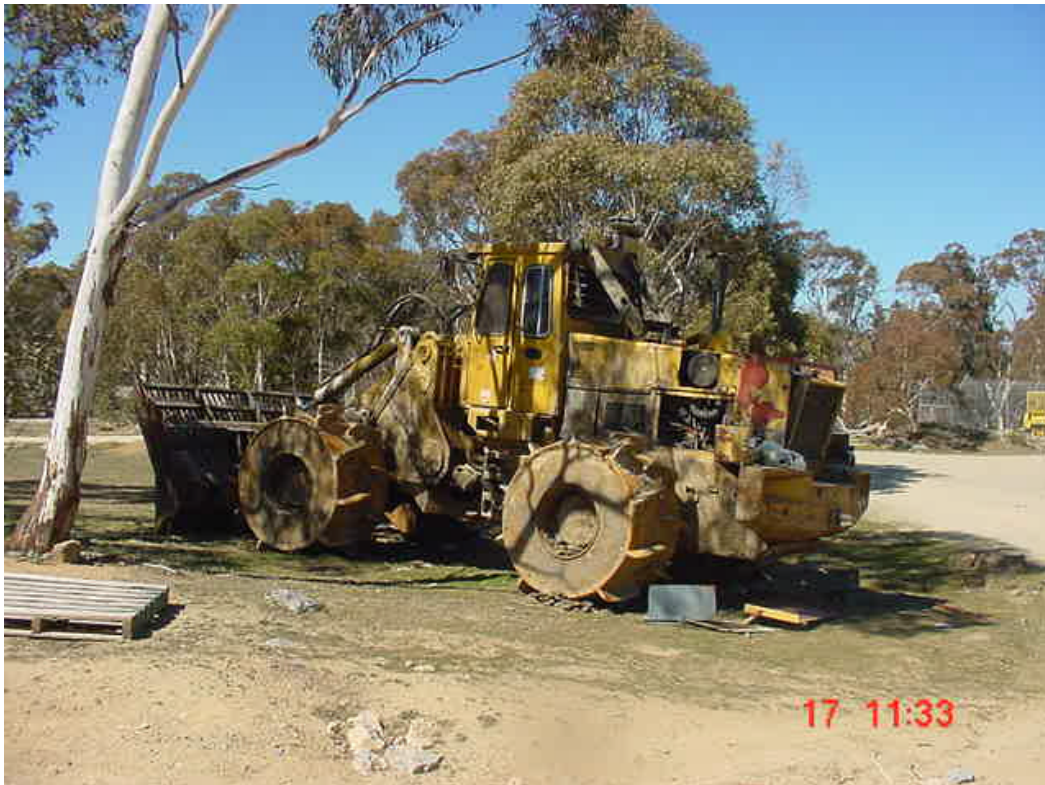
PHOTOGRAPH No.33. Bulldozer / Compactor at Sawpit Creek Landfill
