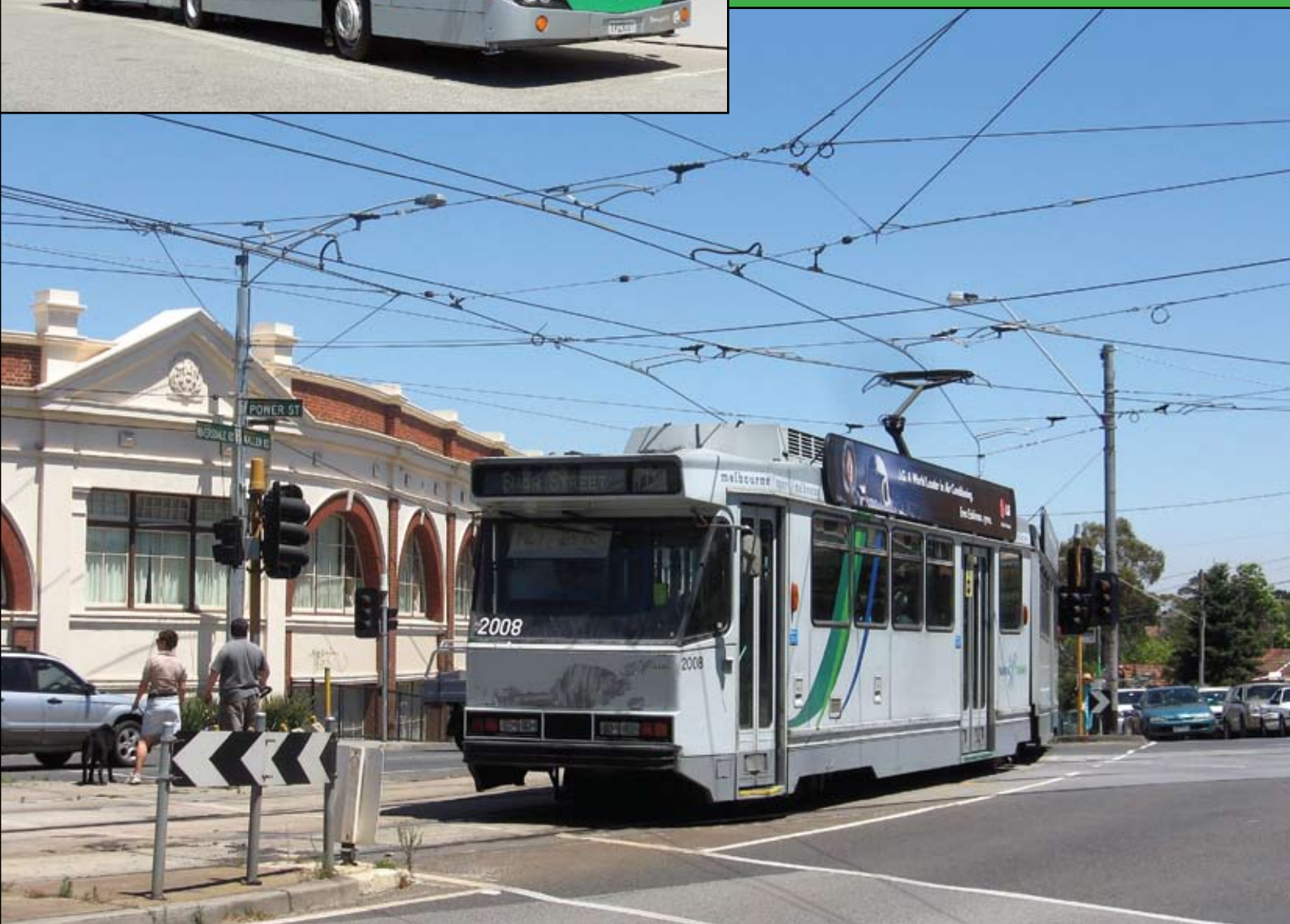
BELOW: On 12 December 2007 Hugh Ballment photographed B2 class tram 2008 in the street outside Hawthorn Depot. Note the mix of trolley bus and tram type overhead with the long hangers and twin pull-offs which is the current Melbourne style of overhead.
