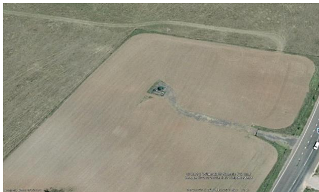
Image D. Access track and well head causing severance to arable land. Note small island of unploughed land outside well site.
