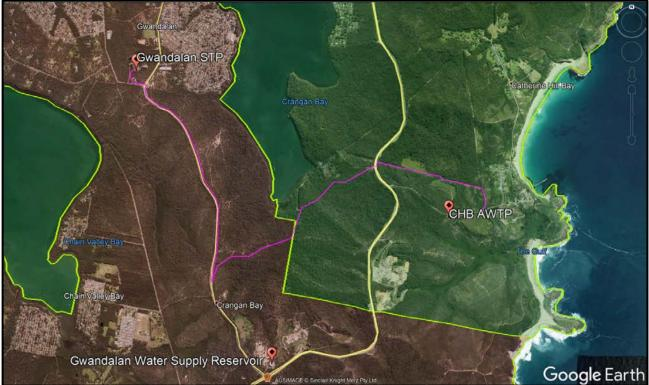
Figure 2 – Proposed SRWTM Pipe Alignment.
