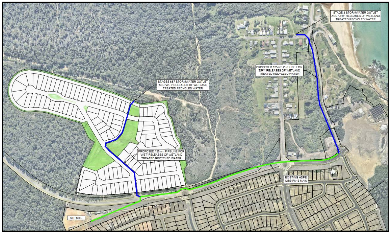
Figure 7 – Proposed pipeline routes to the wetland-treated recycled water 'wet' release location adjacent to the stormwater outlet of Stages 6 and 7, and the wetland-treated recycled water 'dry' release location at Lindsley Street.
