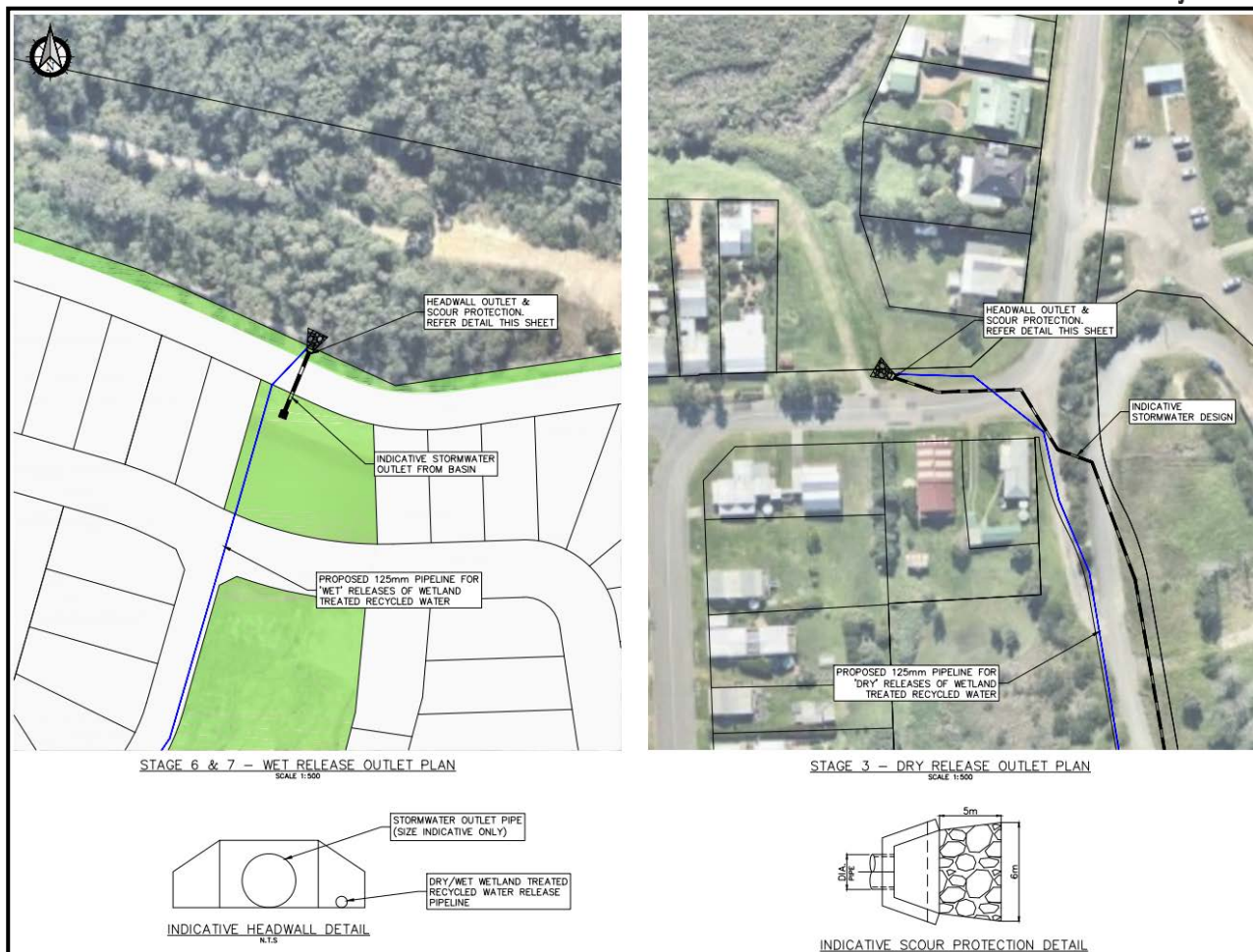
Figure 8 – Concept headwall designs for the wetland-treated recycled water 'wet' release location adjacent to the stormwater outlet of Stages 6 and 7, and the wetland-treated recycled water 'dry' release location at Lindsley Street.
