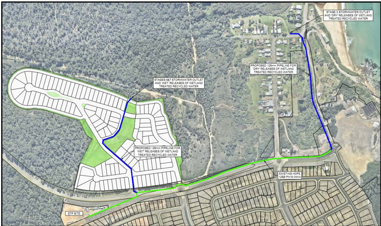
Figure 2: Proposed pipeline routes to the wetland-treated recycled water 'wet' release location adjacent to the stormwater outlet of Stages 6 and 7, and the wetland-treated recycled water 'dry' release location at Lindsley Street.
