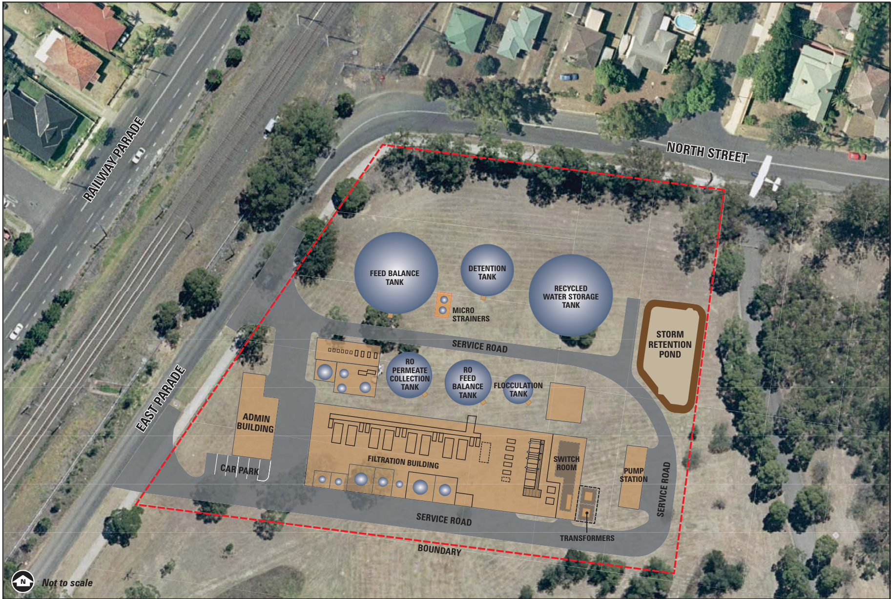
Figure 3-2 Recycled Water Treatment plant detail
